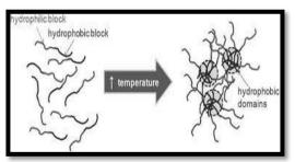
Fig 1: Mechanism of temperature-sensitive system
